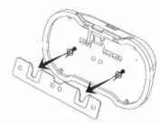
There are two screws at the back of the Peephole Host, then hang them to the right position on the metal plate.
